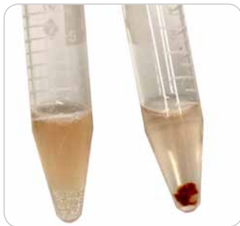
Figure 1. Protein Extraction Beads are required for efficient tissue disruption using the Bioruptor®
