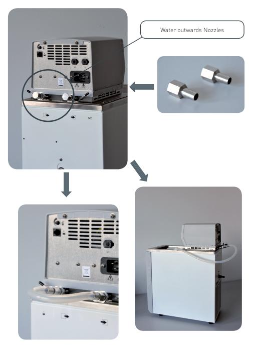
Use spare Tubing (8mm | D x 12mm 0 D) to set a continuous loop up.
