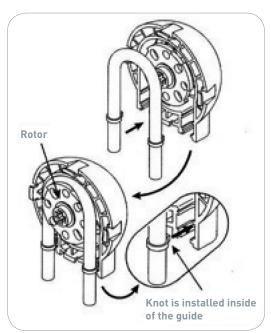
Cut with scissors the silicon tube standing for the warm and cold flow where you want to integrate the pump.
