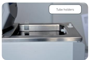
At least, two plastic holders per pipe are required to fix appropriately the pipe because it moves constantly due to peristaltic pump head movement.
