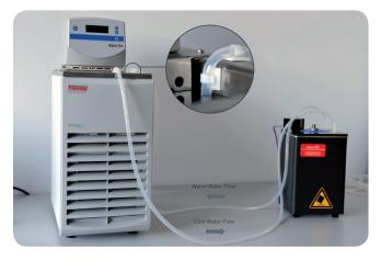
**Note:** submerge the pipe into the cold water reservoir, the end of the pipe must be one cm above the bottom of the tank.
