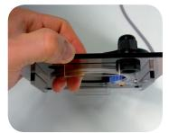
Then, connect the pipes to the *Bioruptor waterbath*. Insert the silicon 6 x 9 mm pipes in the black plastic connectors.
