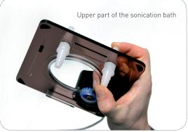
Connect a piece of silicone tube with the lower part of the connecting tool which is connected to warm flow. This piece of tubing will determine the level of water in the Bioruptor's tank as the circulator is "sucking" the water from this opening. This will be done later when the circulator is filled with water. The tubing can be cut gradually with a pair of scissors to allow a progressively higher level of water. The required level is determined by the blue line "water level") in the tank.
