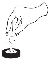
Gently **press** the chip with the **chip positioner** to set a good position
