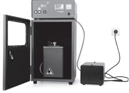
9. Place the control unit on top of the soundproof box. Plug the power cable into the outlet and switch on the power switch on the back of the control unit.
