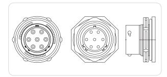
When connecting cables, always be sure pins are properly aligned. Note the indexing pins on the control unit cables for precise mating alignment.
