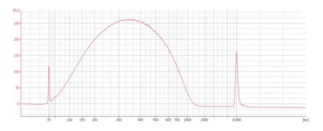
*Figure 1:* Agilent High Sensitivity DNA chip profile of sheared genomic DNA: smear around 400 bp.
