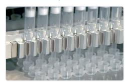
Diagenode's IP-Star system uses the principle of bead-based magnetic separation. Magnetic beads bound with chromatin or DNA are brought to the inner wall of the tip when a strong magnetic force is applied. This differs from other systems that collect the bound DNA on the bottom of a reaction well, resulting in cleaner assays and less carryover.
