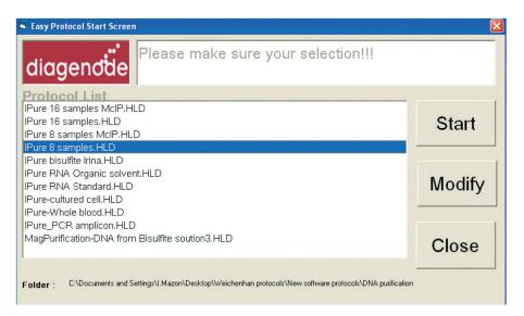
6. Before starting the protocol a start confirmation window will appear. Press OK and the protocol will run.
