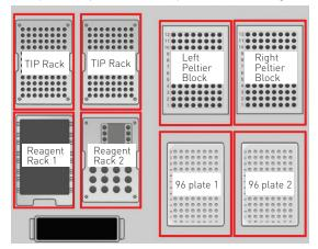
5. Add 2 µl of carrier to each IP and input sample and place them on the Left block.
