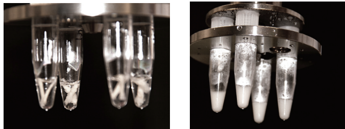
Figure 2. Efficient deparaffinization of FFPE sections by sonication using the Bioruptor Pico.
