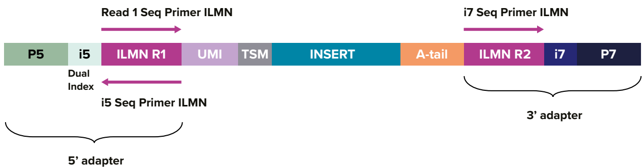
Figure 10. D-Plex cell-free RNA-seq library construct after preparation.
